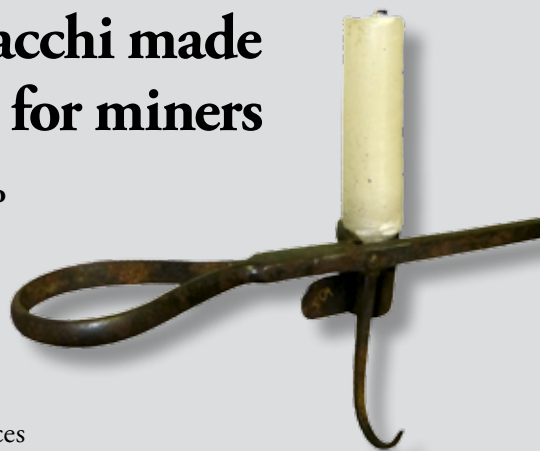
Miners could slide the curved end of the pricket light over a beam. The hook was often used to hang a birdcage or a lunch bucket. And the pointed end could be wedged into a hole or crack in the wall.
